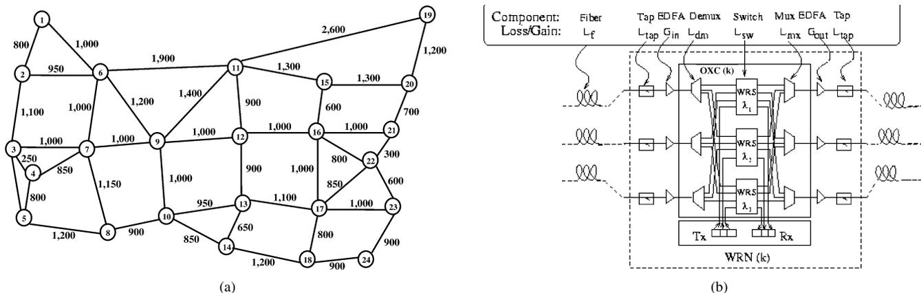
Fig. 1. (a) A sample mesh network with fiber length (in km) marked on each link. (b) Architecture of a wavelength-routing node (WRN) [7].
